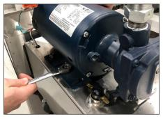
**Step 27:** Using the four bolts, reattach the motor to the caddy frame.
