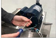
**Step 5:** Remove screws to open wire housing.
