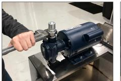
**Step 4:** Disconnect the quick disconnect from the top of the pump.
