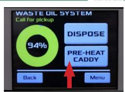
**Step 1:** Push the "Pre-Heat Caddy" button on the control panel.
