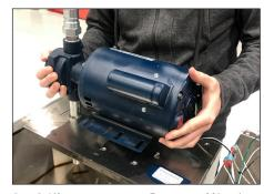
Step 9: Lift to remove motor. Turn motor 90° and set on the Caddy frame.
