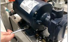
**Step 16:** Using the four bolts, reattach the motor to the caddy frame.
