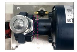
**Step 25:** Reattach the quick disconnect nipple.
