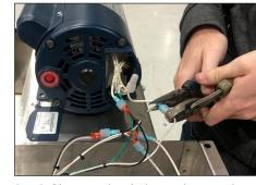
**Step 6:** Disconnect the wire harness by separating the wire disconnect terminals.
