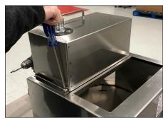
**Step 18:** Resecure the motor housing back to the caddy using the four screws.
