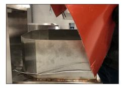
**Step 19:** Put the NEW heater belt in place, being careful to keep belt wires around the bottom of the CURVED assembly.
