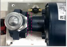
**Step 13:** Begin re-assembly by reattaching the suck pipe and guick disconnect nipple.
