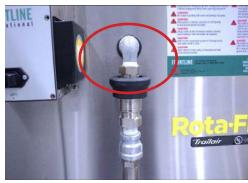
**Step 1:** Connect the caddy hose to the top of the caddy outlet. Then connect the hose to the tank inlet.
