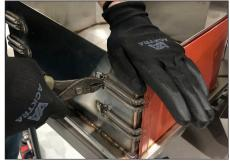
**Step 17:** Using plyers, unclip the springs, four on each **Step 18:** Discard old belt assembly. side of the belt
