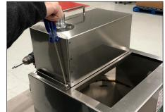
**Step 2:** Remove the four screws in the motor cover housing.
