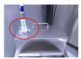
**Step 2:** Connect quick disconnect to top of motor housing.
