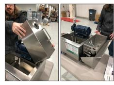
**Step 3:** Remove motor housing, pivot and rest the housing onto the caddy chute in order to take pressure off the wire casing.
