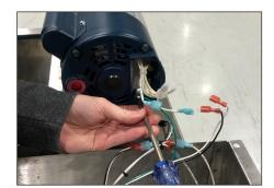
**Step 7:** Loosen the ground wire screw.
