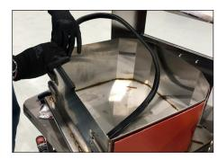
**Step 21**: Once springs are re-attached, re-secure the rubber gasket, starting at the mid-point of the FLAT backside of the Caddy assembly.
