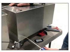
**Step 10:** Remove screws at the base of the caddy bucket.
