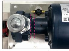
**Step 14:** Begin re-assembly by reattaching the suck pipe and quick disconnect nipple.
