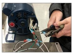
**Step 17:** Connect the wires back to the wiring harness terminals.
