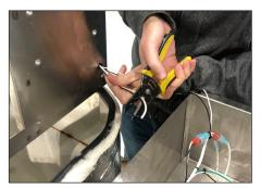
**Step 13:** Cut the heater belt wires and pull the wires back through the Caddy body.
