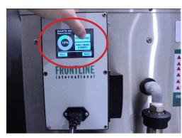
**Step 1:** Push and hold down the Dispose button.
