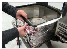
**Step 14:** Carefully remove the tape from the back of the **Step 15:** Remove insulation to expose springs, setting bucket. If tape tears you will need to replace with heavy duty tape or duct tape when re-assembling.
