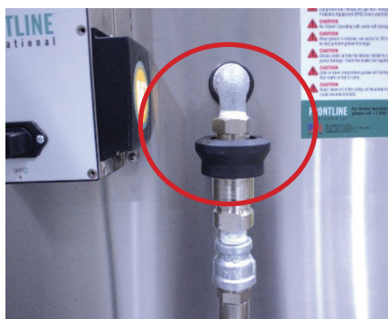
Step 2: Connect the caddy hose to the top of the caddy outlet. Then connect the hose to the tank inlet.
