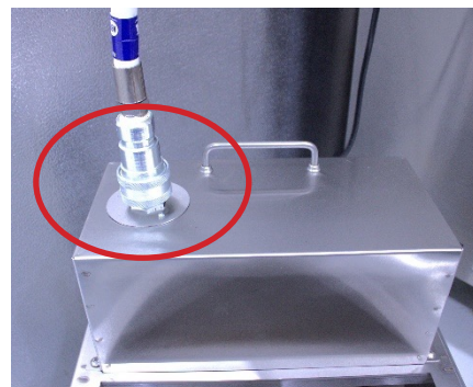
Step 3: Connect the IEC power cord to the caddy electrical housing, then to the front of the control panel.
