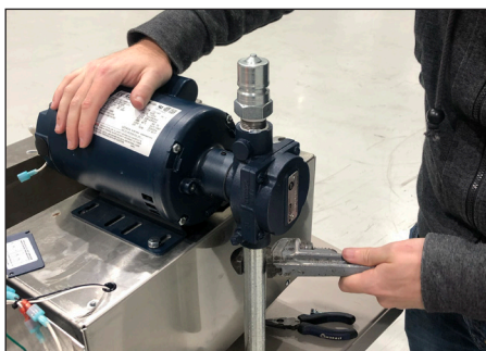
Step 11: Using a pipe wrench, remove the suck pipe from the bottom of the pump.
