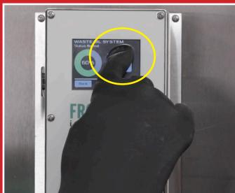
**STEP 9** Turn Caddy motor ON. Press DISPOSE on UCO tank Control Panel. Grease flows to tank.
