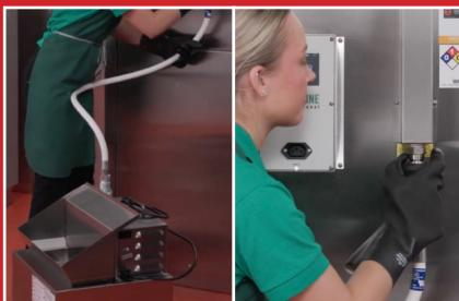
**STEP 8** Connect hose to Grill Grease Caddy body and, other end, to the UCO tank.
