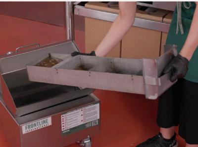
**STEP 2** Pull out the grease drawer and carefully pour it into the Grill Grease Caddy.
