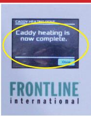
**STEP 7** It's important to preheat the Caddy. On the UCO Tank control panel, choose PRE-HEAT CADDY. There is a progress bar. Screen will alert when pre-heat is complete.
