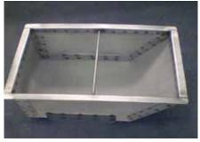
Heated caddy keeps grease from coagulating. Extra-large crumb-catcher basket protects pump and maintains high-quality yields
