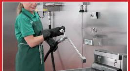
**STEP 5** When vat is empty, **wait 15 seconds**; oil is still moving through the plumbing to the tank.
