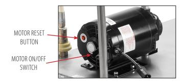
5. Turn the switch on the back of the motor to the ON position.
