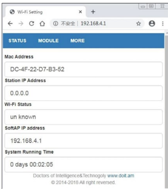
Figure 5.5.3.2 WEB Placement Interface
