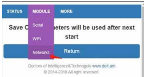
Figure 5.5.3. 13 Entering the Network Configuration Interface
