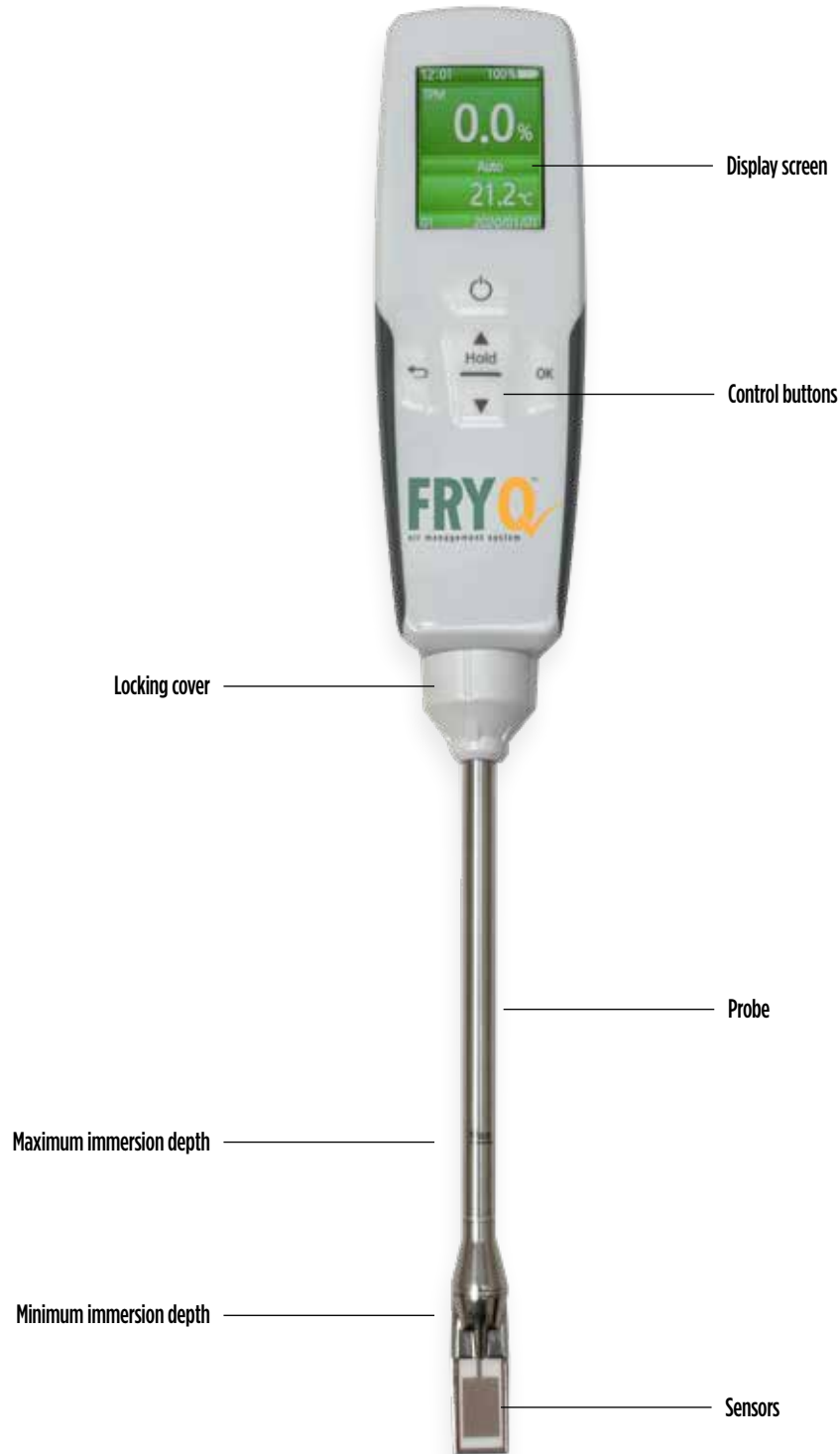
Figure 2.1.1: Front view of the FryQ instrument
